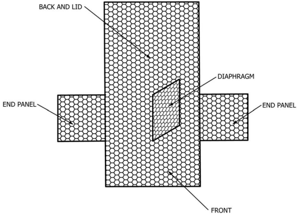
Figure 2: Mechanically Manufactured Gabion
