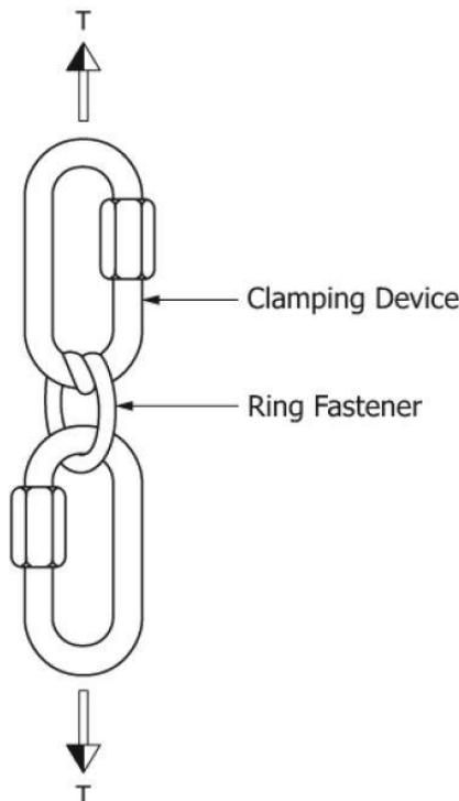
Figure 5: Single fastener test with load applied perpendicular to the closing axis
