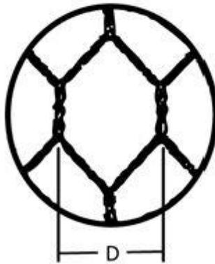
Figure 4: Wire mesh opening nominal dimension *D*
