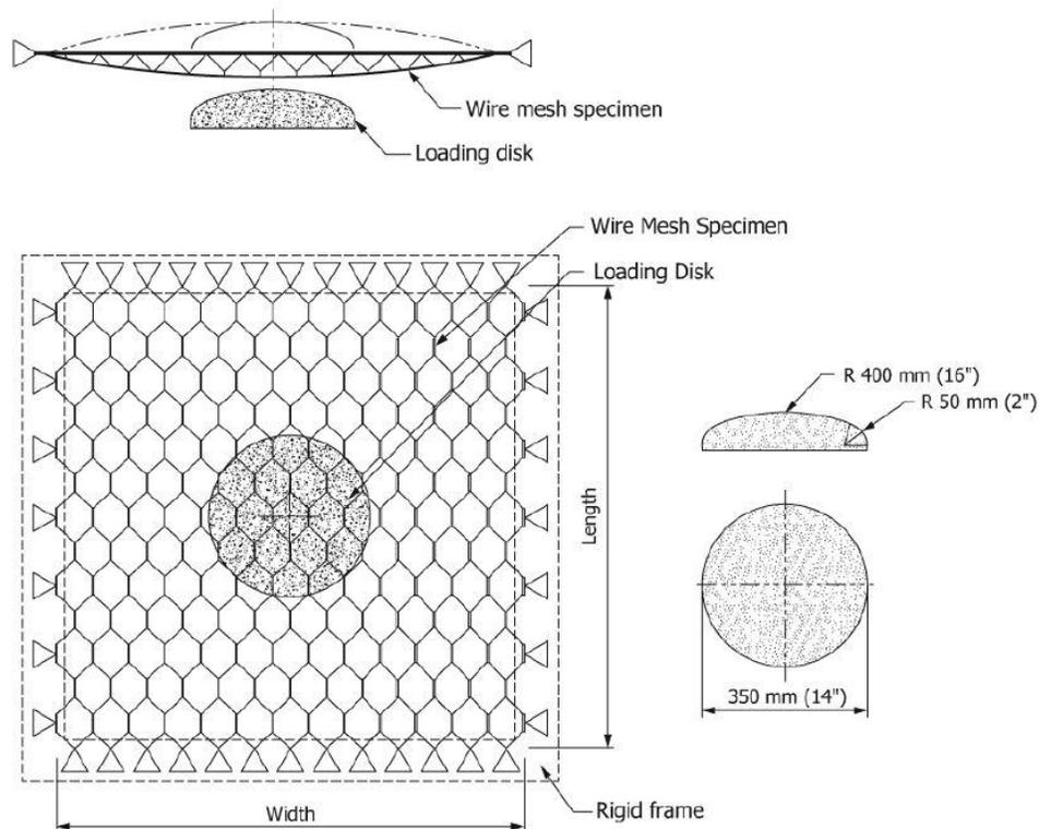
**Figure 6: Secured punch test with every mesh clamped**
