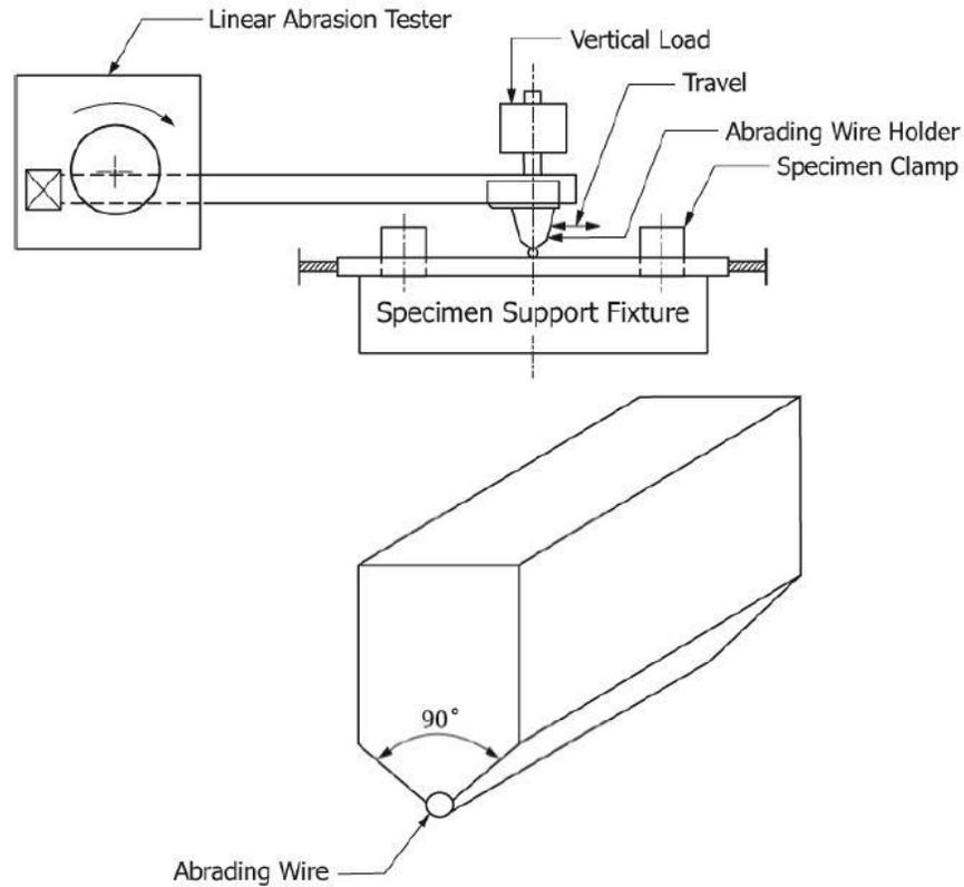
Figure 7: Linear abrader
